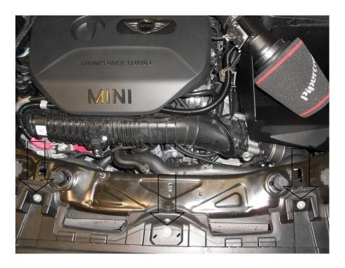
9. Unclip the sensors at each end of the crash bar and remove the foam crash bar cover.
