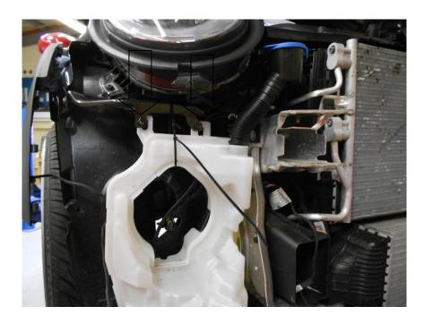
18. Using a flat blade screwdriver or similar remove the 2x clips inside the wheel arch. Using T27 Torx driver undo the 1x screws. Lift the duct upwards to release it and remove it from the vehicle.
