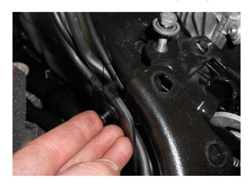
22. Undo the 2x radiator pins using a screwdriver or T30 Torxs driver.
