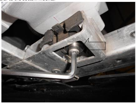
30. Before securing the radiator to the intercooler check that the bracket and locating peg are correctly engaged on the fan shroud.
