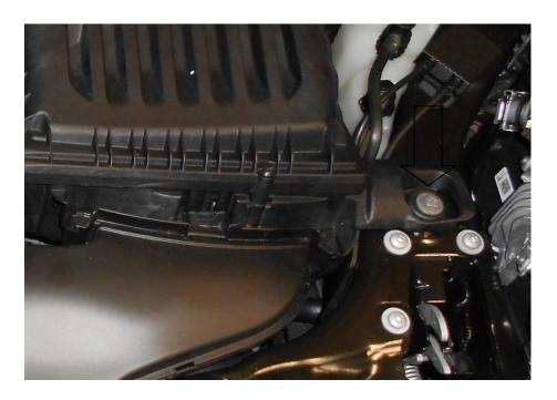
21. Using a flat blade screwdriver or similar tool remove the 1x plastic clip on each side.
