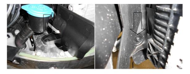
14. Using a 13mm socket and suitable ratchet undo 2x bolts on either side of the crash bar. Pull the crash bar forward and remove it from the vehicle.
