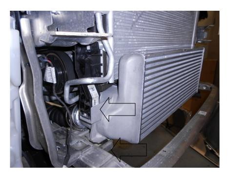
29. Using the 2x M8x16mm Allen cap bolts and 2x 8mm Penny washers supplied secure the intercooler to the bottom mounts.
