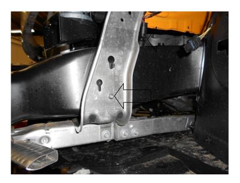
17. To access the bolt for the other duct you need to move the washer fluid reservoir. Using a T30 Torx undo the 2x bolts lift the reservoir upward to release it from its bottom mounts. To support the reservoir cable-tie it to the bracket above.
