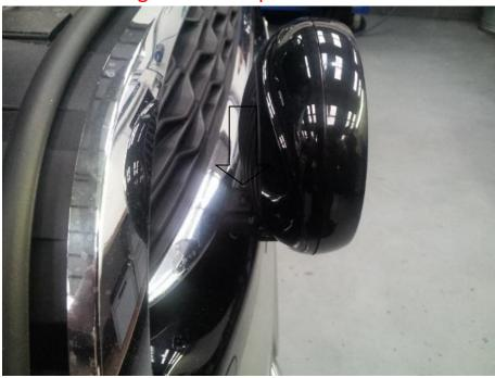
8. Undo the 3x T30 Bolts across the top of the bumper. You will require a second person to carefully pull the bumper forward and clear of the vehicle. Store in a safe place to prevent it becoming damaged while carrying out the rest of the installation.
