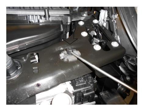
23. Undo the 2x T30 Torx screws on either side of the intercooler. Using a flat blade screwdriver or similar tool carefully release the spring-clips and disconnect the hose at each end of the intercooler.
